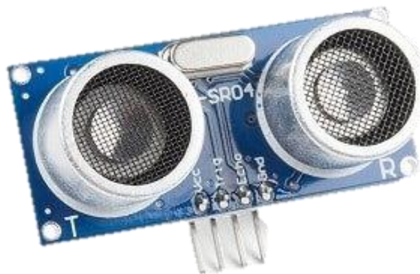
Figure 33. HC-SR04 Ultrasonic Sensor
