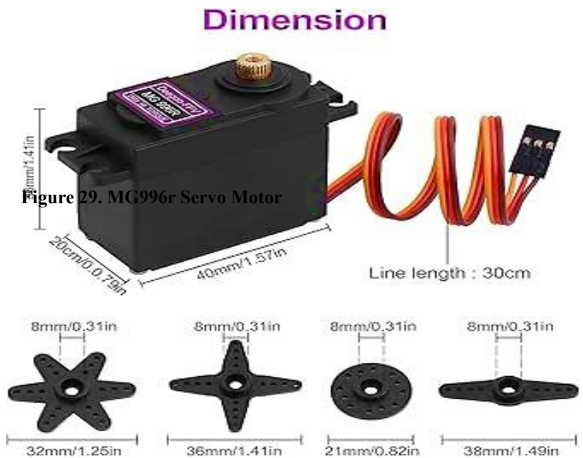
Figure 27. MG996r Servo Motor
