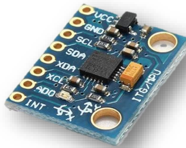
Figure 32. MPU6050 GY-521 Sensor
